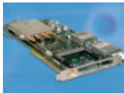
ECOTEL® ISA 4 xx plug-in card with 4 GSM-, CDMA or UMTS channels
